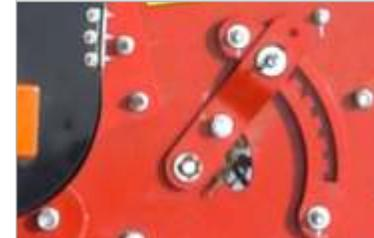
A mechanically adjustable rotary agitator ensures additional gentle sieving on the second main web. Thus, the sieving performance is increased, especially under heavy digging conditions.
