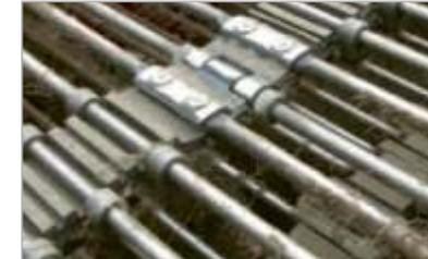
For changing conditions: The main webs of the SGWR 200 are fitted with web joiners with wear bushes. This extends the life of the web and allows for easy and quick changing of web sizes when conditions demand it.
