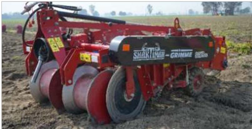
Tractor Mounted Machine, with Hydraulic Cylinder second web folding for improved handling and manoeuvrability on headland
