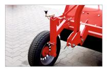
The support wheels are equipped with a spindle for stepless height adjustment. in addition, pendular support wheels can be selected, which allow steering movements.
