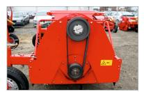
The 4-fold V-belt drive ensures an even transmission of the required torque.
