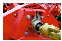
The freewheel in the drive train reduces the load on the PTO shaft and the drive shafts when disengaging at the headlands.
